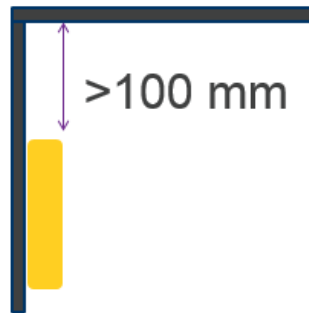
Figure 21: Keep Air Interface away from nearby metals
