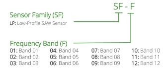
When commissioning a system, care must be taken not to duplicate same sensor frequency bands within a given asset. IntelliSAW recommends selecting sensors based on their groupings for optimal performance. Please contact sales for more details.
